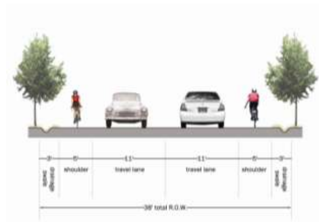
Figure 3: Diagram of shoulder bike lane
