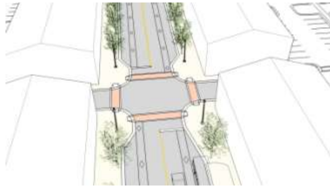
Figure 8: Urban Complete Street intersection design
